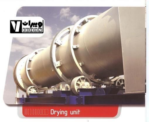
The aggregates are fed by the dryer feed belt into the lower part of the dryer drum in which the initial section contains a series of spiral flights which feed the material towards the internal flights. The flights have been designed in such a way as to lift the aggregates and then drop them in a thin veil in front of the burner flame ensuring an efficient drying process. The Drying unit is started through Siemens soft start technology, resulting in a smooth activation process.
